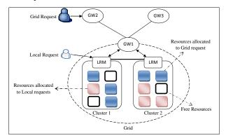
Fig. 1. A scenario that shows the contention between local and external requests in a resource sharing environment
